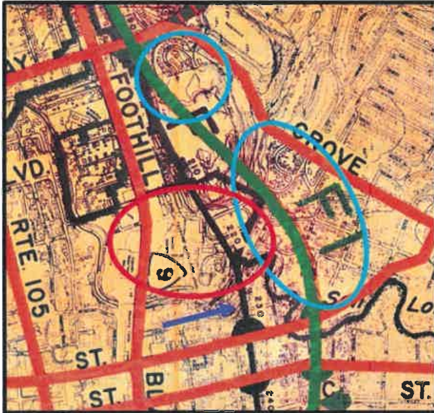
Figure 1: Highway Planning Map for the Foothill Freeway: The original route laid out by the State engineers was the “F” line, shown here in black (blue arrow). It ran almost entirely south of Castro Valley, but bisected the old, no longer used Hayward High School athletic fields (red oval). Hayward leaders succeeded in getting the route pushed north to nearer the F1 line (Green), which now ran through Ruby Meadow (teal oval).
