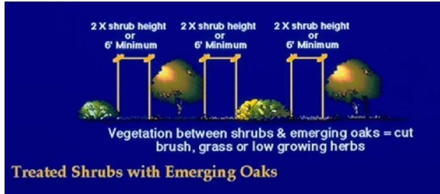
Figure 18. Shrub island spacing. Design groups of plants small enough to provide horizontal separation between groups. This allows proper maintenance and helps slow the spread of fire. Each shrub or group of plants should measure no wider than two times its height, or less than 120 square feet (or 6 feet x 20 feet). The space between groups should be greater than three times the height of the shrubs.
