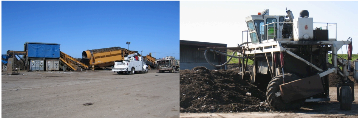
Figure 1: Photos of noise-generating equipment similar to those proposed for the Jess Ranch composting facility. The machine shown in the right photo is the mobile "compost turner". The left photo shows the stationary equipment consisting of the yellow "trommel screen" on the right feeding material into the "pre-screener/horizontal shredder" beneath the blue tarp on the left. The horizontal shredder is used to grind wood-like material such as palm branches, etc. The ground material then drops into the two debris boxes below. The useful output from the material-handling equipment is discharged back onto the compost pile by means of the conveyor system seen to the extreme left of the left photo.
